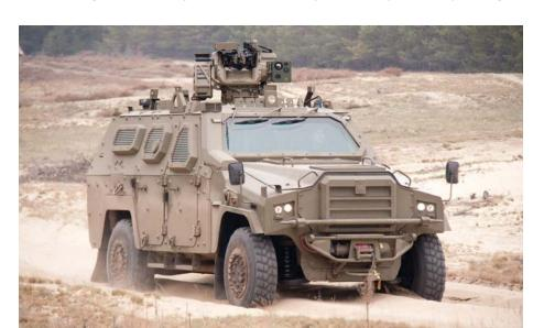
all-round field of vision to the commander irrespective of light or weather conditions. The vibration-resistant container comprises a daytime zoom camera (30x optical, 12x digital zoom) with a colour and a B/W modes. At night or in unfavourable conditions, a continuous-zoom cooled thermal camera is used. Distance measurement are performed by an eye-safe laser rangefinder which can reach up to 25,000 m. The commander sight's elevation range is between -90° and +70°.
